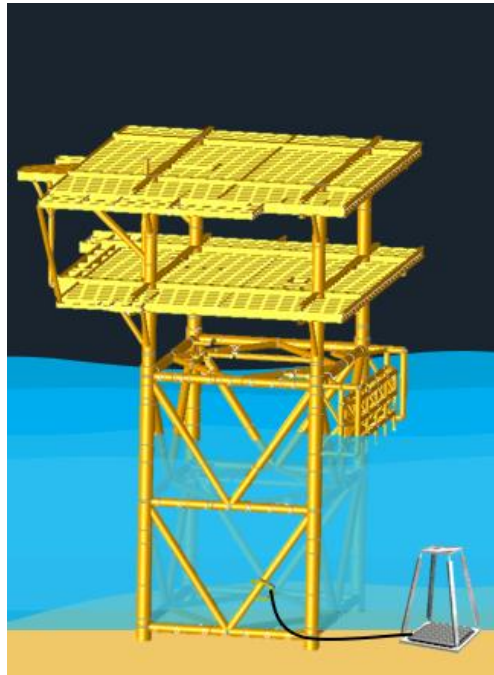
4 Legged Anodepod Cable connection is prone to theft
