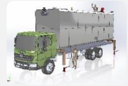
Temporary mobile tank to support inspection & repair
